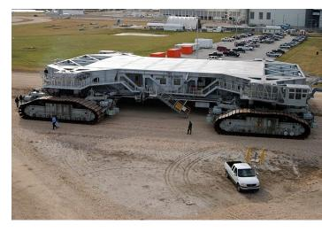
3.4 miles may seem like a drop in the bucket compared to a trip to the moon, but this journey came with its own logistical challenges. After assembly at the Vehicle Assembly Building, the Saturn V rocket was loaded onto the largest self-powered land vehicle in history, a Crawler-Transporter, and then moved to the launchpad at a snail's pace of one mile per hour.
